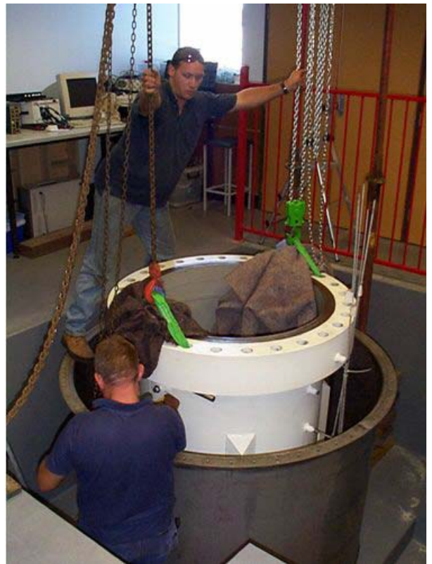
Lowering the Chamber into the Temperature Controlled Tank
